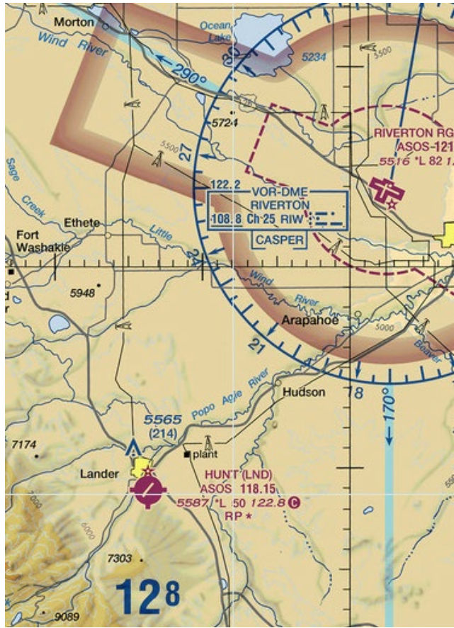
Figure 3-10: Class E Airspace in vicinity of Lander, WY Starting at 1,200' AGL with Class G Uncontrolled airspace to the surface below.
