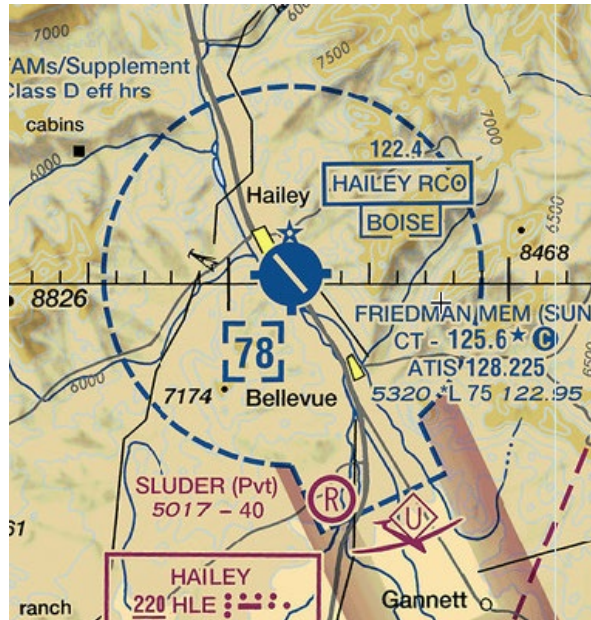
Figure 3-6: Class D Airspace – Sectional Chart Depiction Class D is depicted by a dashed blue line surrounding a blue, towered airport symbol.
