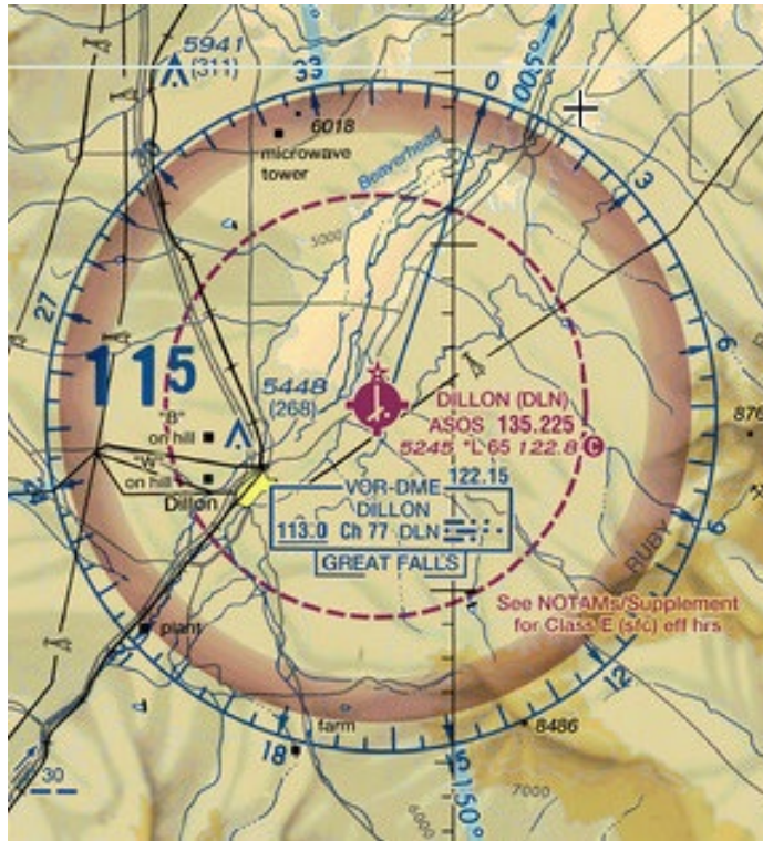
Figure 3-8: Class E Airspace Designated to the Surface by a Dashed Magenta Line
