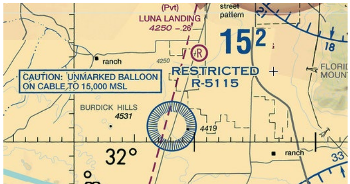
Figure 4-4: Example of a Tethered Aerostat Radar System and Sectional Chart Image of Moored Balloon Hazard Area.
