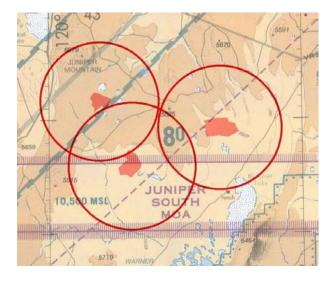
Figure 6-11: Solution to Overlapping TFRs
