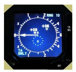
2. **Terminal Collision Avoidance Device (TCAD)** is a low cost anti-collision system detecting and alerting pilots to nearby IFF transponder-equipped aircraft but not providing evasive instructions or coordination with other aircraft. ADS-B (IN) will provide improved data.
