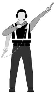
To inform the flight crew of the airstairs moving away from the aircraft, the parking tender will utilize the **Airstairs Removed Hand Signal**.
