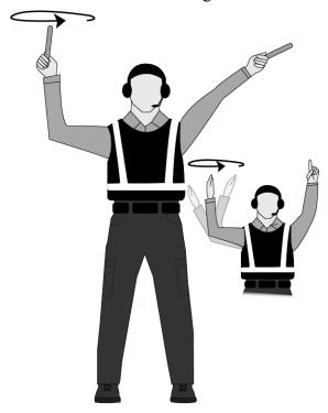
\*Flight crews use numbers (number of fingers held up in the windscreen) to identify the engine to be started. Aircraft engines are numbered right to left from the parking tenders view (left to right from the crew's point of view)—i.e., for an airplane that has two engines, the left engine from the parking tender's point of view is #2 and the right engine is #1.
