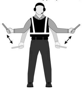
To request the flight crew to set the aircraft brakes, the parking tender will utilize the **Apply Brakes Hand Signal**.
