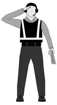
To inform the flight crew not to move flight controls (in the case of an obstruction), the parking tender will utilize the **Do Not Move Controls Hand Signal**.
