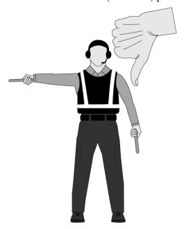
When responding to the flight crew request to connect external power, the parking tender will utilize the **Connect Power Hand Signal**.
