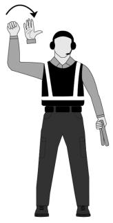
To inform flight crew of chocks inserted or flight crew requesting chocks, the parking tender will utilize the **Chocks Inserted Hand Signal**.
