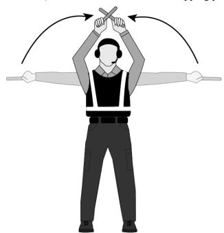
To stop an aircraft in the event of an emergency or possible collision, the parking tender, or wing walker will utilize the **Emergency Stop Hand Signal**.
