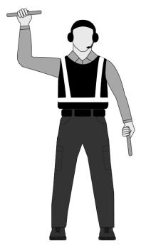
To inform crew of loss of radio communication, the parking tender will utilize the **Loss of Communication Hand Signal**.
