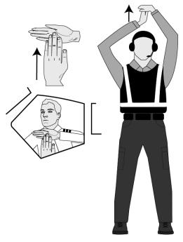
When responding to the flight crew request to disconnect external power, the parking tender will utilize the **Disconnect Power Hand Signal**.
