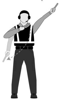
To inform the flight crew of end of marshalling, the parking tender will utilize the **End of Marshalling Hand Signal**.
