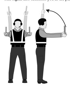
To move an aircraft forward in a straight line, the parking tender will utilize the **Move Forward Hand Signal**.
