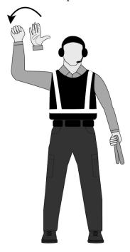
To request the flight crew to release the aircraft brakes, the parking tender will utilize the **Release Brakes Hand Signal**.
