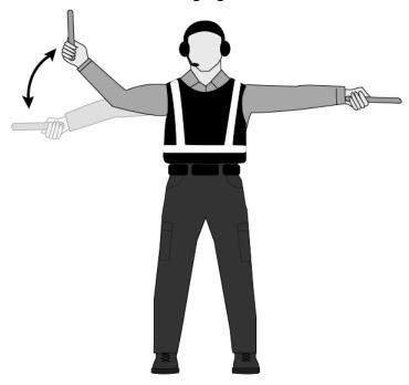
To stop an aircraft normally, the parking tender will utilize the Normal Stop Hand Signal.
