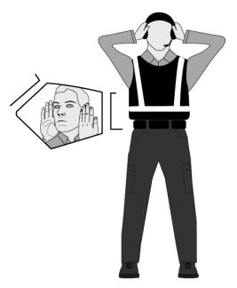
To inform the flight crew of an engine or brake fire, the parking tender will utilize the **Fire Hand Signal**. \*This is an emergency signal and should be repeated over the radio.\*
