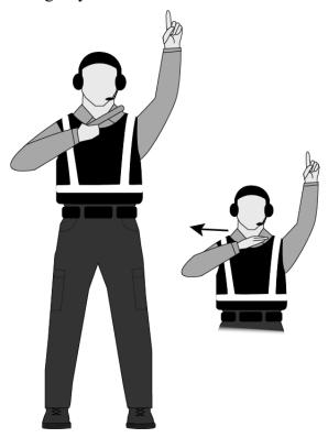
The proper signal for a stationary wing walker is wand (or hand with thumb up) extended above the head. If the aircraft comes within an unsafe distance of an object, the wing walker will utilize the Emergency Stop Signal and/or radio call until the operation stops.
