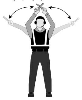
To pass control of marshalling off to another parking tender, the parking tender will utilize the **Next Marshaller Hand Signal**.
