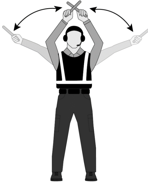
Figure 6: Emergency Stop Hand Signal
