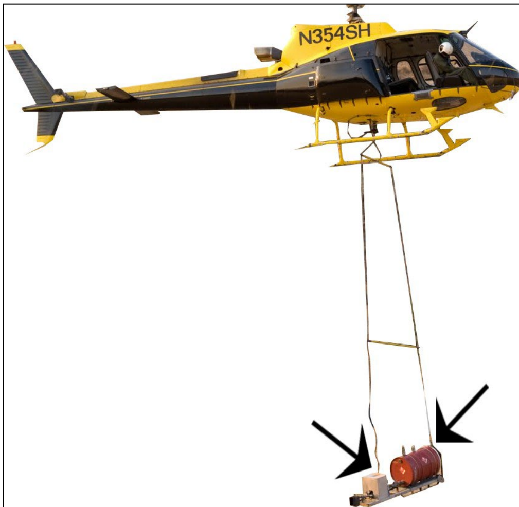
Figure 3. Location of Attachment Points of Single Point Cable Assembly
