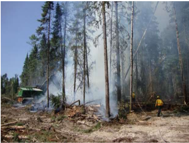
Figure 7.23. Wildfire caused by failure of a hydraulic hose on feller buncher.
