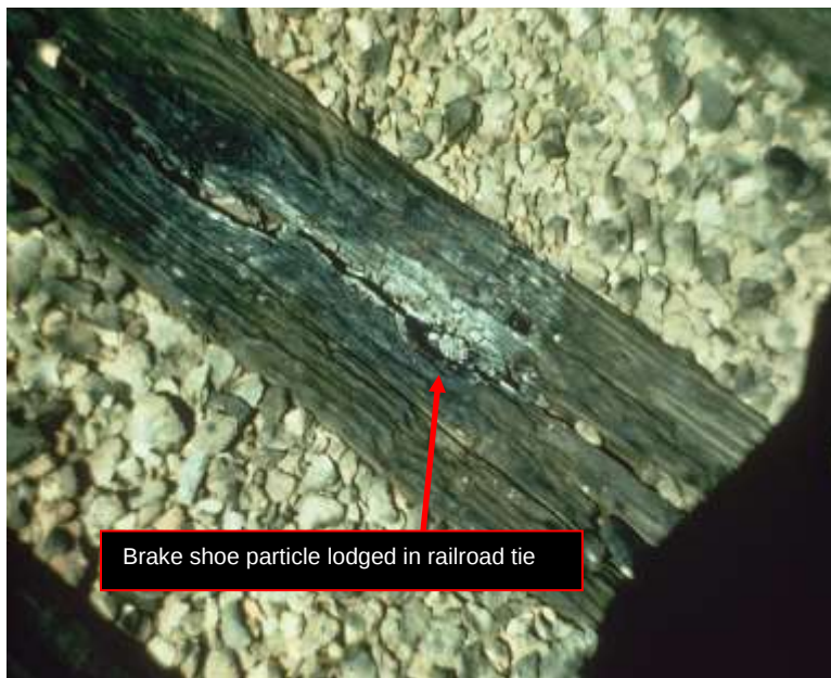
Figure 7.76. Brake shoe particle in railroad tie.
