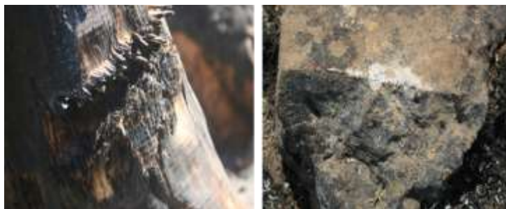
Figure 7.20. Examples of rubbing and impact friction ignition.
