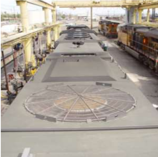
Figure 7.79. Dynamic brake grid exhaust outlet.
