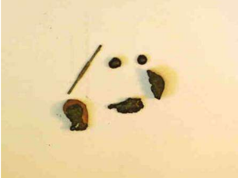
Figure 7.28. Welding byproducts recovered from fire scene.
