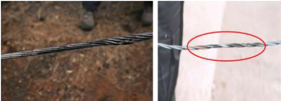
Figure 7.50. Blowhole near tree from electrical grounding.
