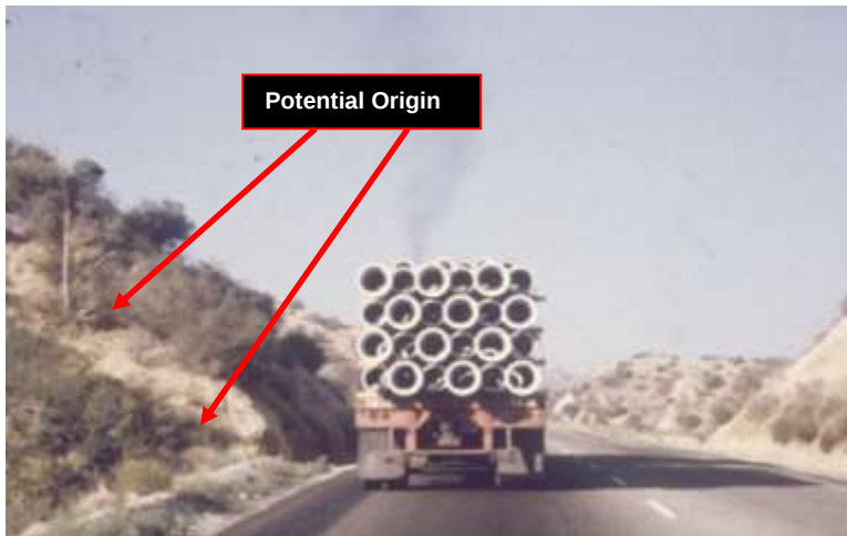
Figure 7.14. Vegetated cutbanks can form receptive fuel beds for exhaust particle fires.
