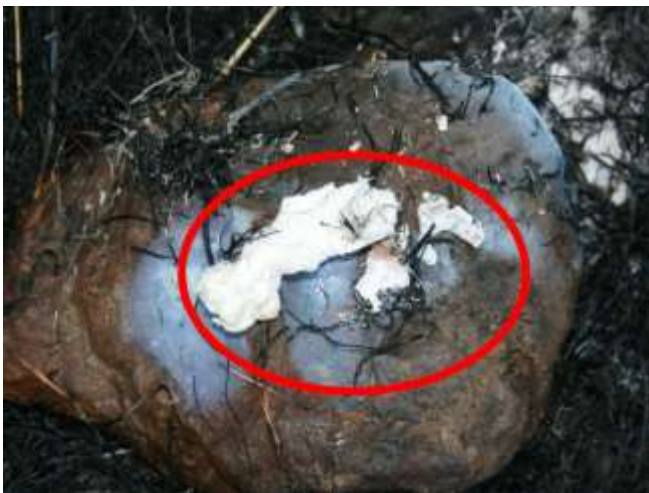
Figure 8.8. Slag from fusee on rock.
