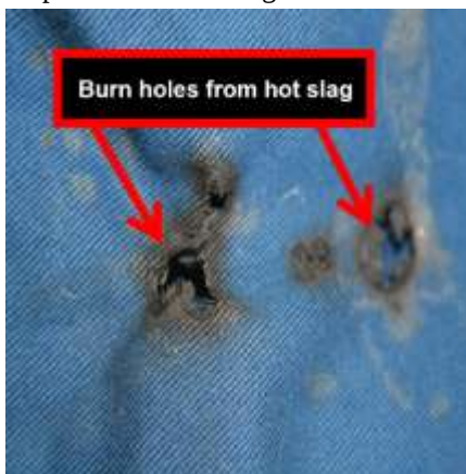
Figure 8.11. Burn holes on pant legs of suspect from fusee slag.
