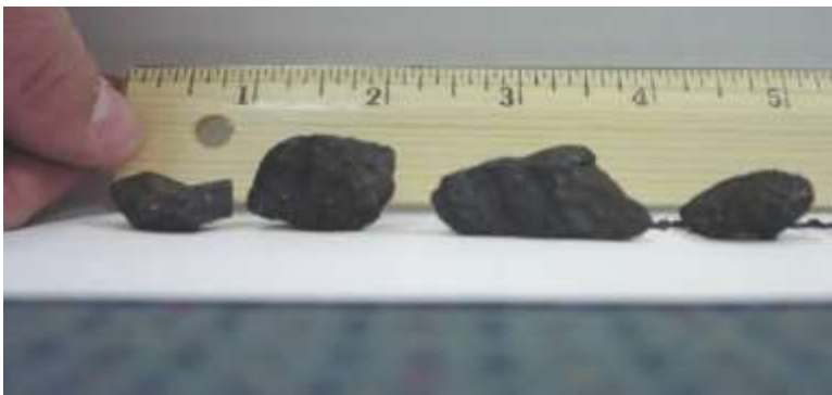
Figure 7.74. Sizes of railroad exhaust particles.
