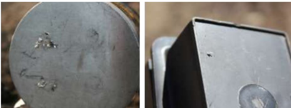
Figure 7.22. Friction particles found by using a magnet.
