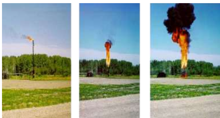
Figure 7.66. Flare stack malfunction leading to ground fire.
