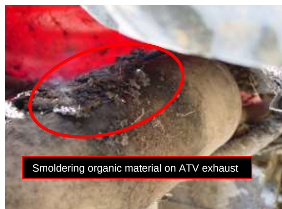
Figure 7.25. Conductive heat transfer ignition factor.
