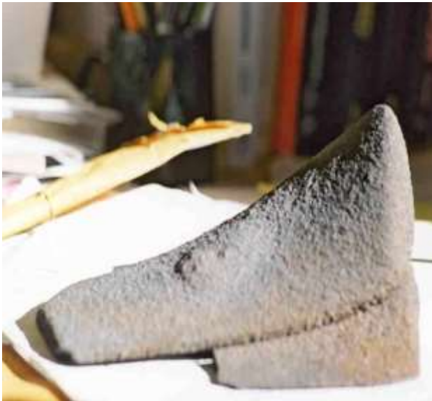
Figure 7.78. Track grinding slag.
