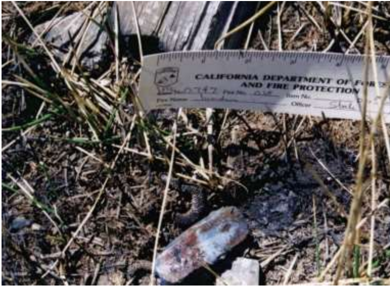
Figure 7.85. Roller bearing thrown from wheel assembly that was hot when it landed in the vegetation as exhibited by the burned area around it and under it.
