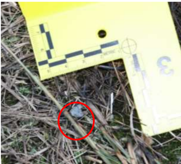
Figure 7.19. Catalytic converter particle.
