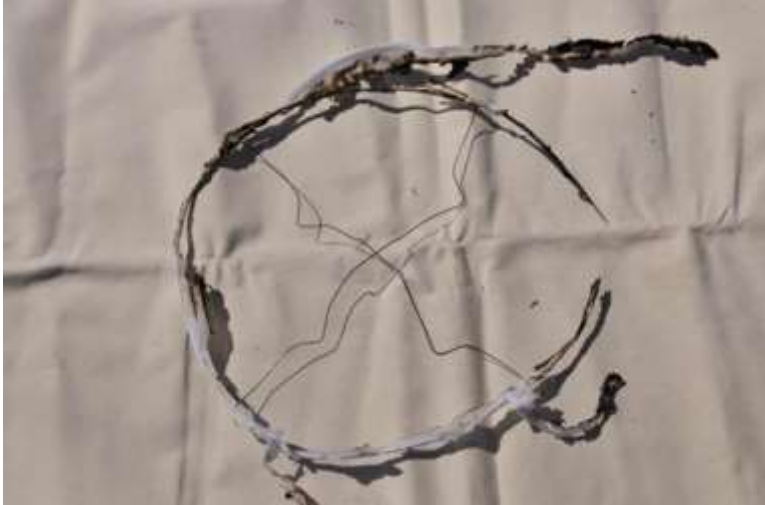
Figure 7.88. Remains of flying lantern after burning.
