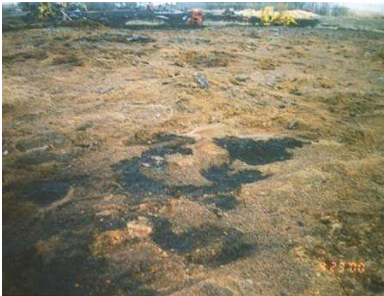
Figure 7.94. Typical fire effects in sawdust or wood chips when spontaneous combustion occurs.
