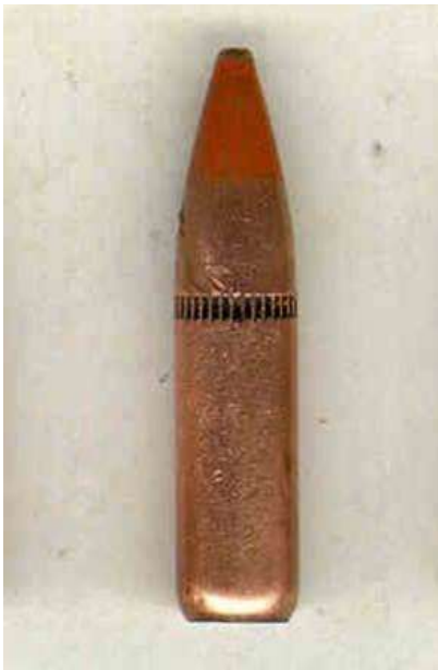
Figure 7.33. Orange tip marking of tracer round.
