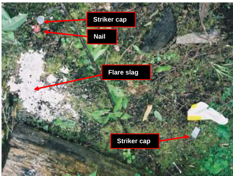
Figure 7.80. Signal flare debris.
