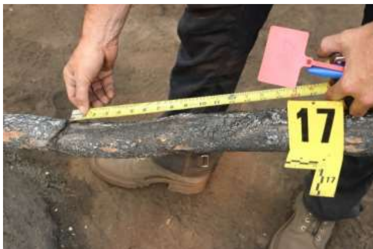
Figure 7.48. Limb damaged by contact with an electrical conductor.
