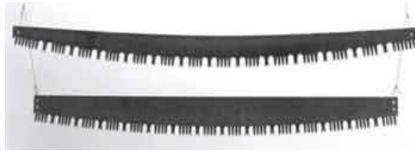
Figure: Comparison of felling and bucking saws.
