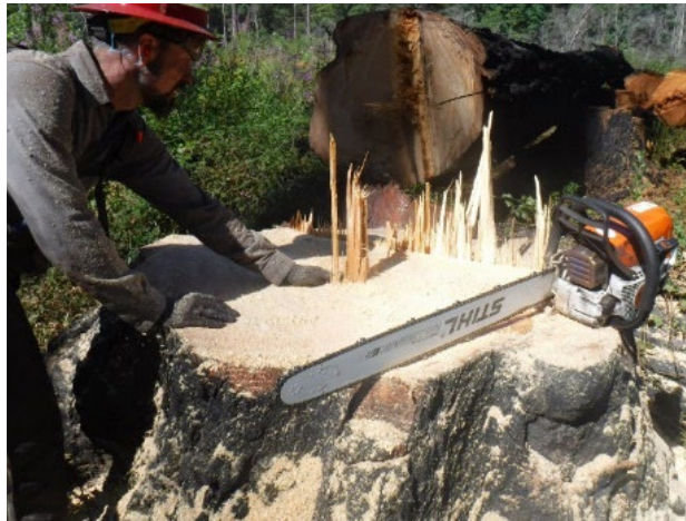
Figure: When developing your cutting plan minimize the amount of walking from side-to-side to reduce exposure and finish the backcut from the best side of the tree.
