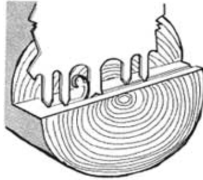
Figure: How a crosscut saw cuts.
