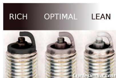
The color of the spark plug's porcelain tip can indicate how the mixture is burning. A white colored plug shows a lean mixture, where a dark plug shows a rich mixture. A light brown color is optimal. Inspect the plug for running condition after jetting changes and evaluating the engine performance by ear and feel.
