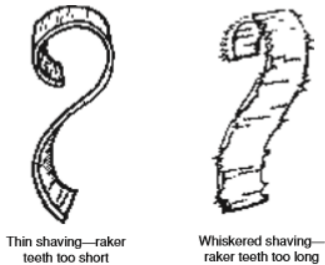
Figure: Examine shavings to identify sharpening problems.
