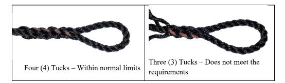
Figure 3—Comparison of a compliant splice that has four tucks with a non-compliant splice that has three (3) tucks.
