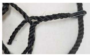
Figure 2—Example of a rope end that has been braided past the splice and tucked underneath a different strand. Note that the splice has four (4) tucks.
