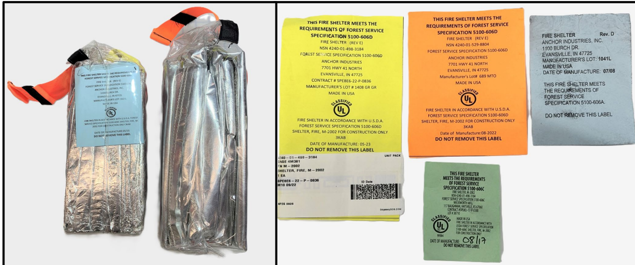
Figure 6: Left image shows missing insert label on non-specification shelter. Right image shows different specification label sizes and colors.
