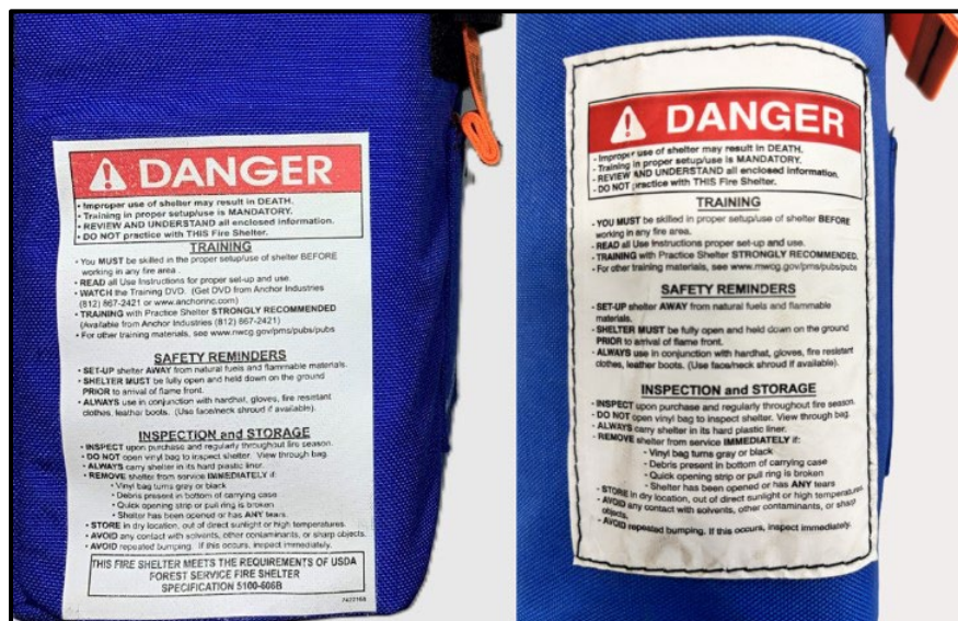
Figure 3: Left is a specification carrying case with heat pressed label, right is a non-specification carrying case with stitched on label.
