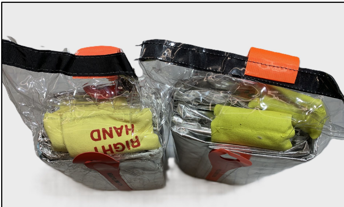
Figure 8: Specification shelter on left, non-specification on right. Note missing stenciling on non-specification shelter.
