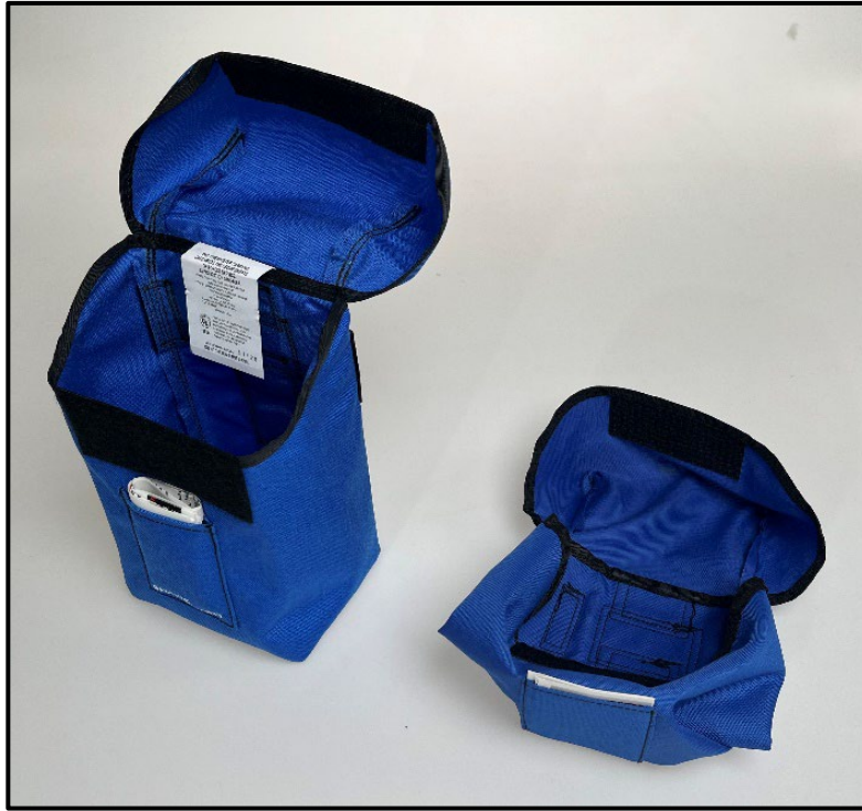
Figure 4: Specification on left, non-specification on right. Note the non-specification case is missing the label and is unable to stand on its own.
