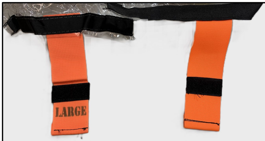
Figure 5: Specification shelter (left) with stenciling, non-specification (right) without stenciling.
