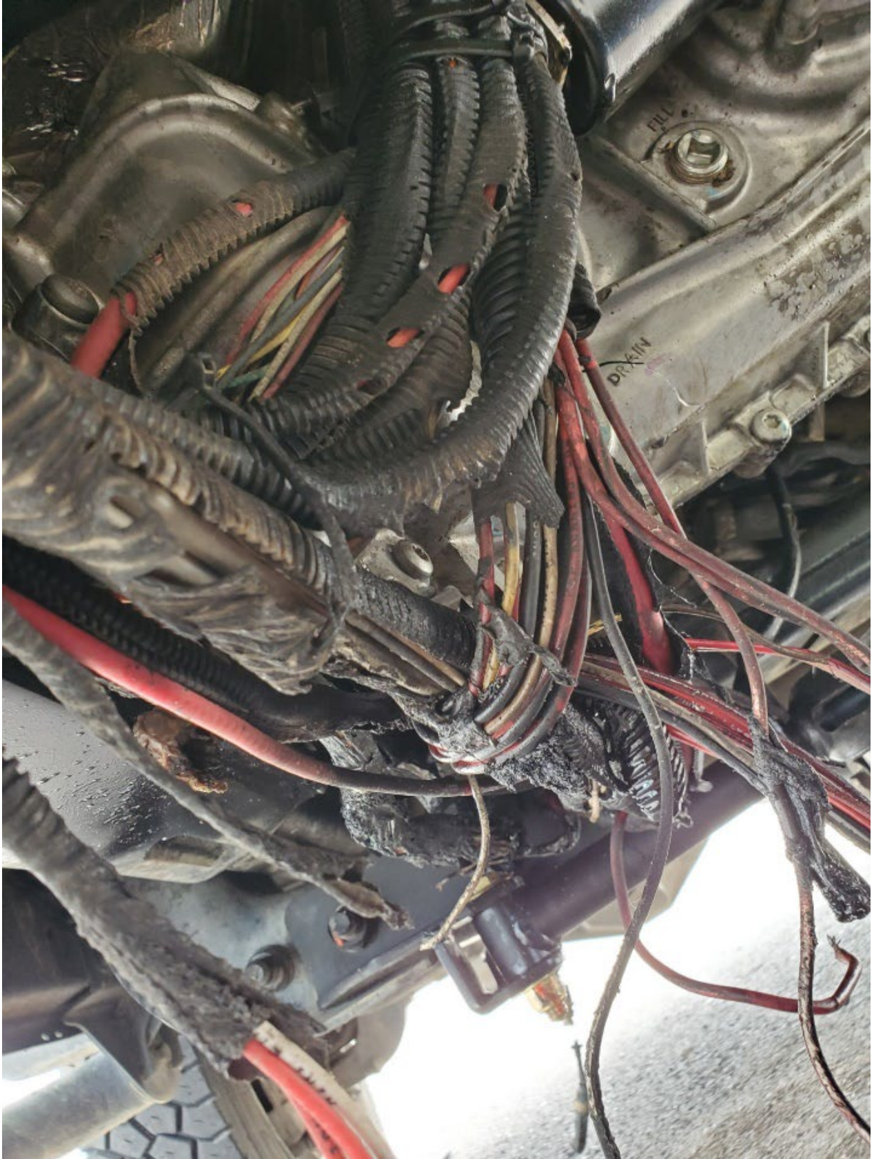
Figure 4: Photo of damage after driveline joint failure.
