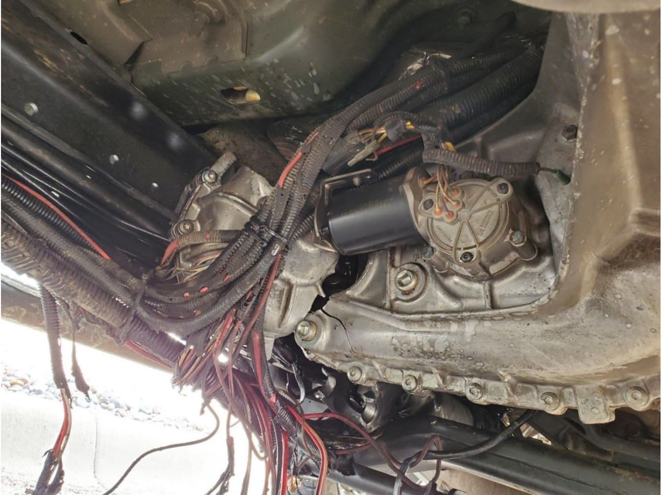
Figure 5: Photo of damage after driveline joint failure.
