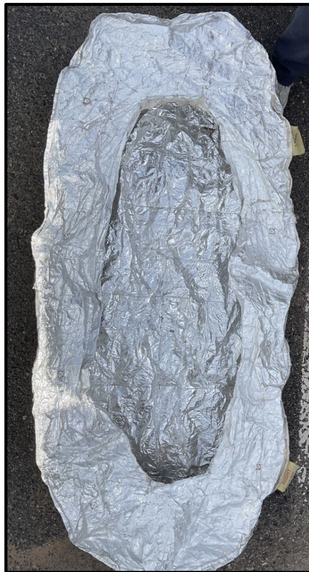
Figure 6: Bottom view, shelter manufactured 2017, minimal indicators of direct heat/flame exposure.
