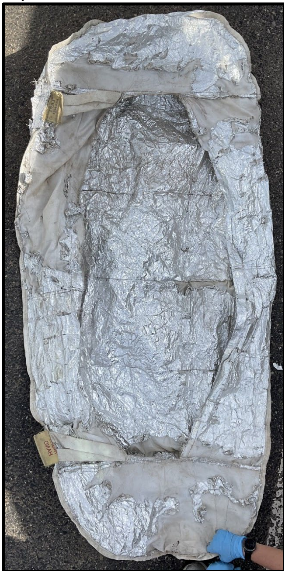
Figure 5: Bottom view, pre-2006 shelter, degradation and delamination present, minimal indicators of direct heat/flame exposure.
