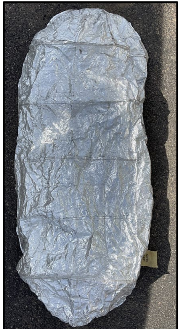
Figure 4: Top view, shelter manufactured 2017, minimal indicators of direct heat/flame exposure.
