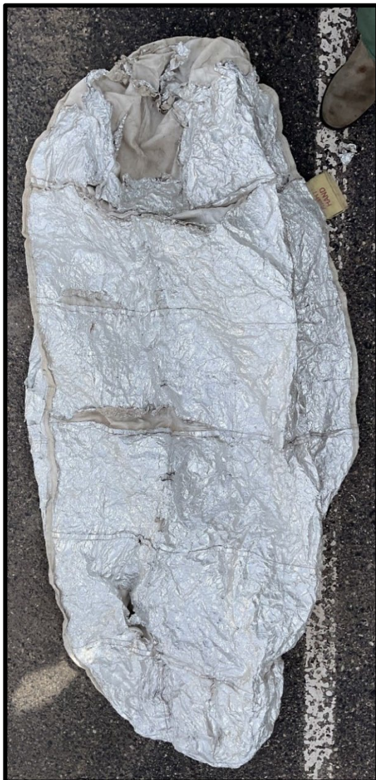
Figure 3: Top view, pre-2006 shelter, degradation and delamination present, minimal indicators of direct heat/flame exposure.
