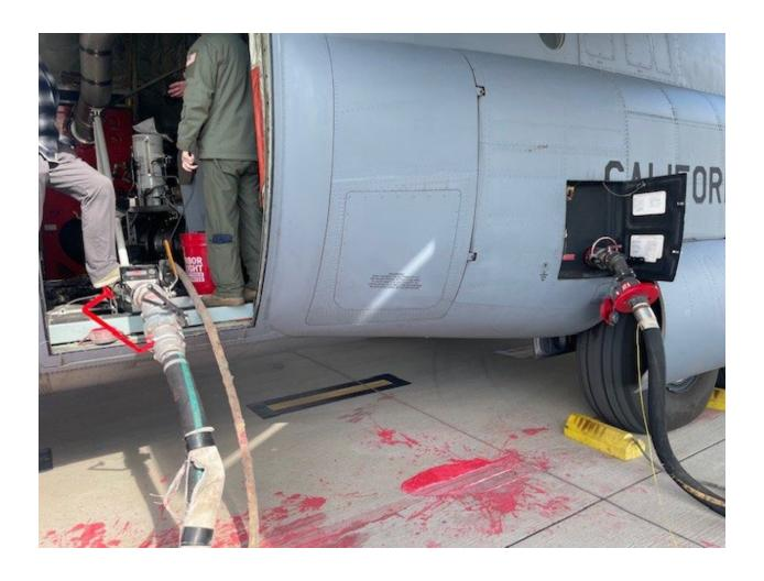
MAFFS C-130 models can only be loaded on the right side of the aircraft. Same side simultaneous fueling and loading can be completed safely by ensuring the fuel truck is positioned such that the fueling hose is not routed under the wing of the aircraft and that the fueling and loading hoses never cross.
