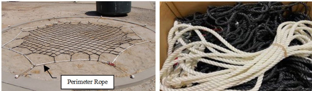
Figure 2—Sample of NFES #000531 cargo net with perimeter rope attached correctly.
