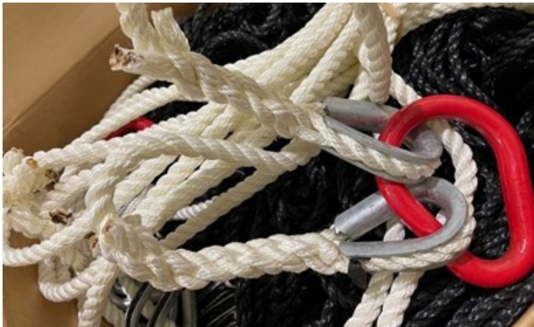
Figure 3—Sample of a correctly manufactured net with perimeter rope strand ends “heat cut” to eliminate fraying.
