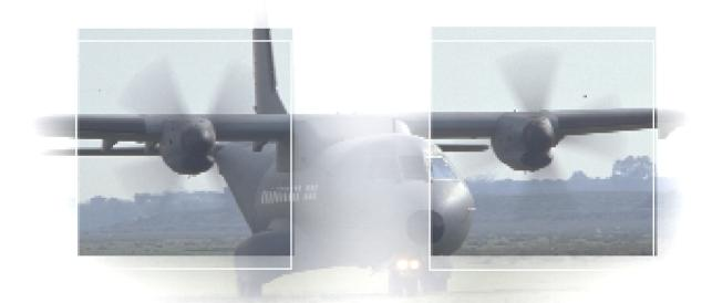
• The rotation of the left-hand side propeller can be stopped with the engine running, on ground only, in order to use the engine's gas generator machinery as an APU, to obtain bleed air for air conditioning, and electrical power by means of the starter generator.
