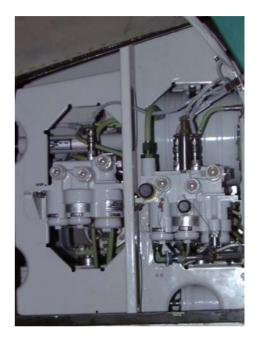
• Two hydraulic accumulators provide pressure to the brakes in case of hydraulic power failure.
