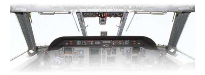
• The distance between crew and aircraft centerline allows good accessibility and visibility to the pedestal and overhead panel for both pilots.
