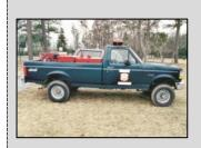
Type 7 Engine Min. Gallons: 50 Min. Flow: 10 GPM Min. Pressure: 100 PSI Min. Personnel: 2
