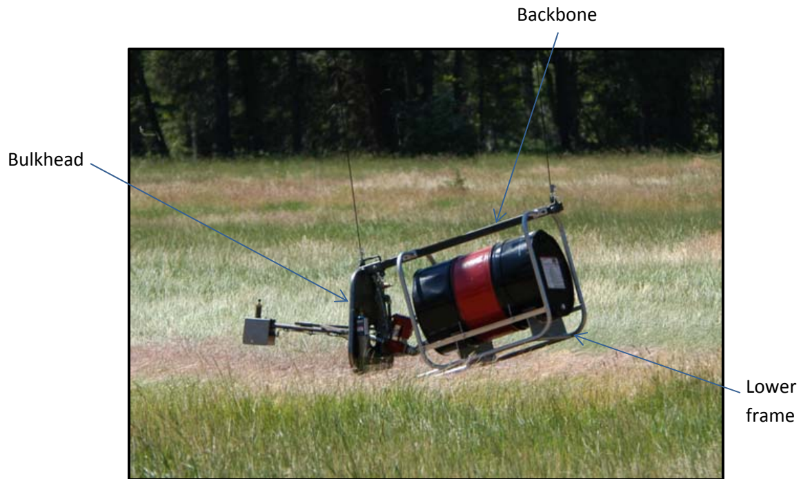
Figure 2. Backbone concept configured as a standard helitorch. The lower frame holding the barrel is connected to the backbone and bulkhead.
