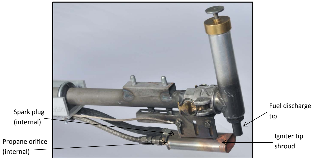
Figure 9. The fuel discharge tip and igniter shroud with the larger protective wind screen removed.
