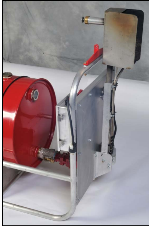
Figure 10. The igniter arm is shown in the raised position. Removal of one push-lock pin releases the arm for use.
