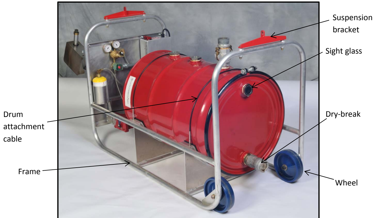
Figure 5. Tank and frame components on the MTDC helitorch.
