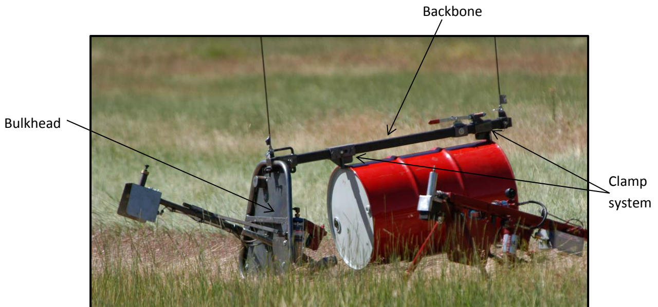
Figure 1. Backbone concept configured as a barrel helitorch with a clamp system on the backbone. A Northern Helitorch frame is sitting in front of the barrel.
