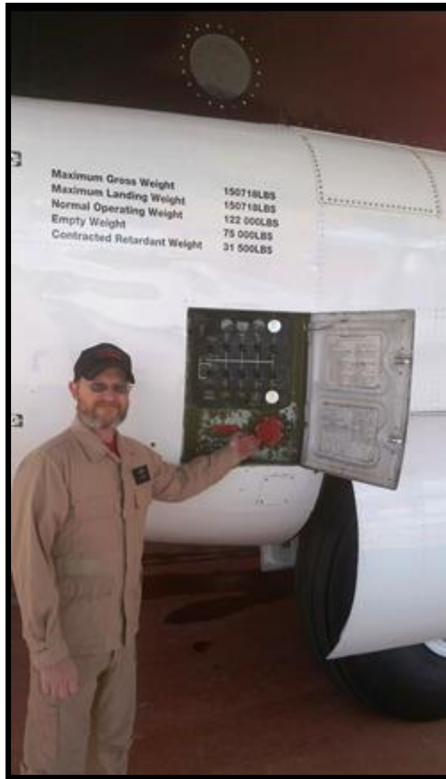
Figure 13 C-130 Single Point Fueling Station
