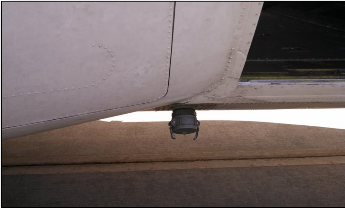
Figure 1 Loading Port Cap C-130
