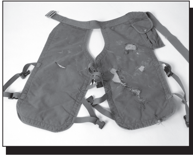
Figure 3—Retire chaps when they have numerous holes and cuts.
