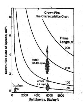
Figure 4b: Fire behavior calculated from models displayed on fire characteristics chart - crown fire driven by the downburst winds.
