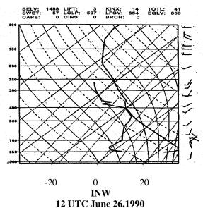
Figure 3: Radiosonde soundings from Winslow, AZ at 1200 GMT on June 26, 1990 exhibiting a classic inverted "V" profile.
