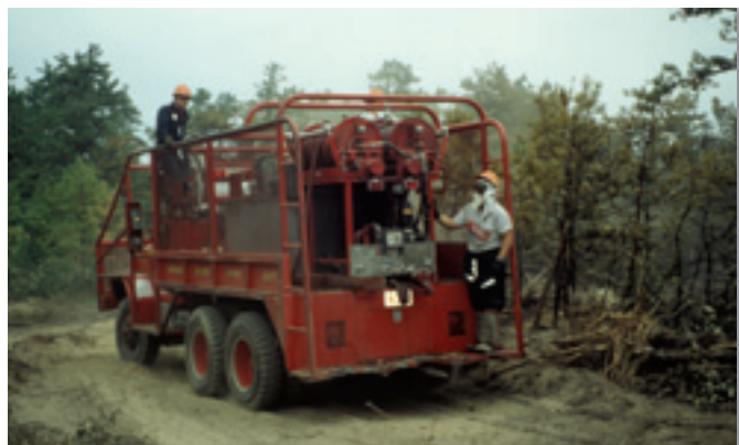
Figure 21—Following safe practices at all times can help reduce fire fatalities. Riding outside an engine is not a safe practice.
