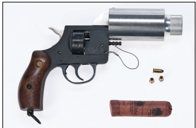
Figure 4–2—A FireQuick flare launcher, 22-cal power loads, and a FireQuick flare.
