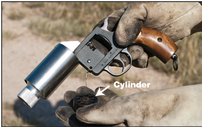
Figure 4-4—To load the FireQuick flare launcher, remove the cylinder.
