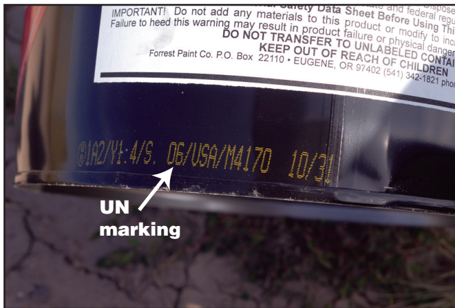
Figure 6–2—Transport blivets in a UN 1A2 steel pail or another container that meets DOT specifications.
