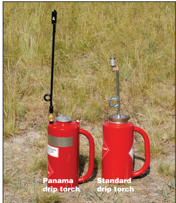
Figure 3–3—A Panama drip torch and a standard drip torch, both configured for transport and storage.
