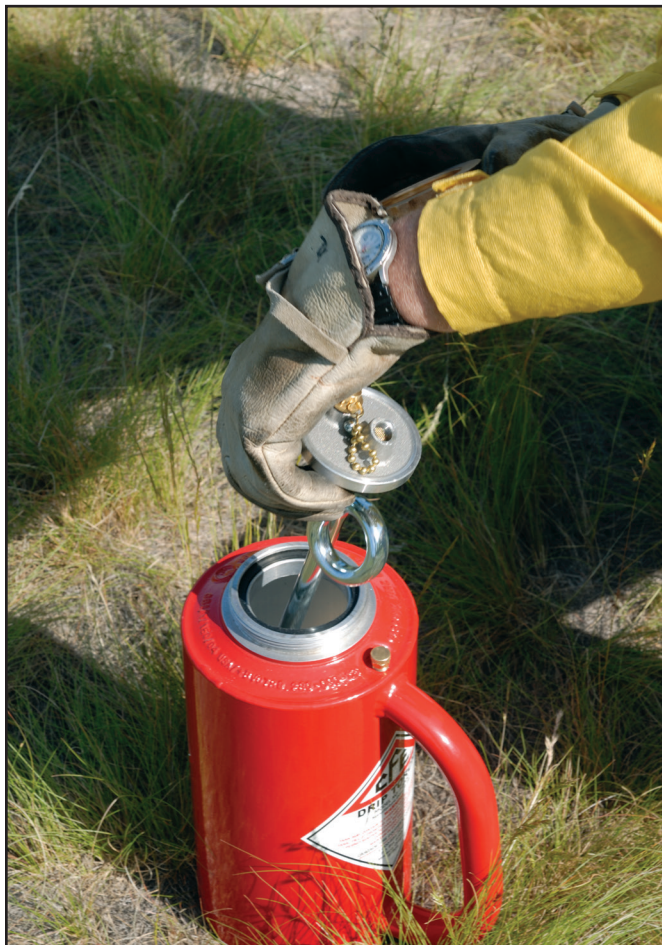
Figure 3-18—Install the tank cover with the fuel spout and wick assembly stowed inside the tank.
