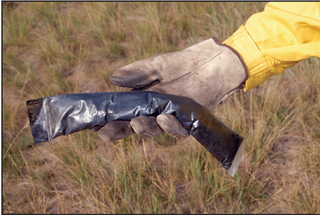
Figure 6–1—This commercially available blivet is called a FireSnake or Heat Source Slash Burner.
