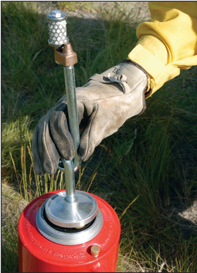
Figure 3–15—Install the tank cover with the spout ready for use.
