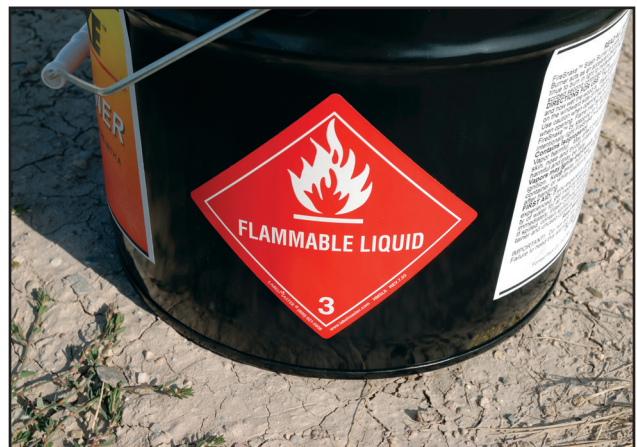
Figure 6–3—Make sure a FLAMMABLE LIQUID label is installed on pails used to carry blivets.
