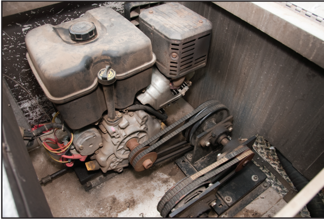
Figure 10–3—Inspect the pump drive belts (if present) for damage and wear. Adjust the tension as needed.
