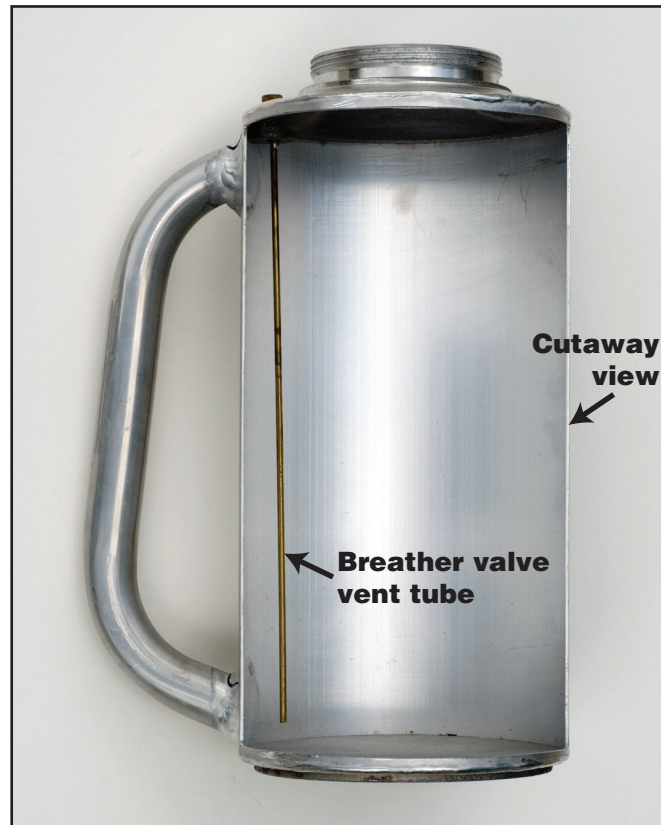
Figure 3-8—Remove the tank cover so you can look inside the tank to verify that the breather valve vent tube is installed and that it has not been damaged. If the vent tube is missing, fuel can pour out of the breather valve and catch fire when the torch is used.
