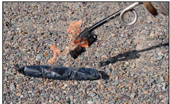
Figure 6-5—Blivets can be ignited with a drip torch.
