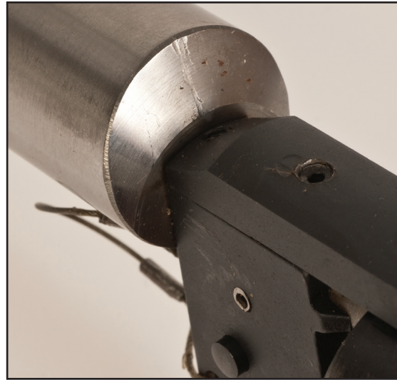
Figure 4-14—This is an example of a FireQuick flare launcher that does not have epoxy sealing the barrel.
