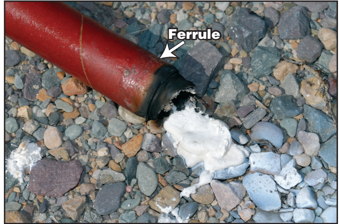
Figure 5-8—Allow fusees to burn completely. The ferrule usually does not burn completely.
