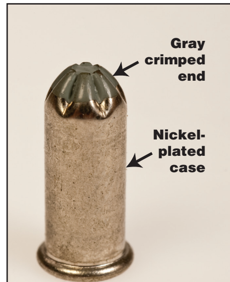
Figure 4-9—A No. 7 power load. The crimped end of the nickel-plated case is painted gray, indicating the power of the load.
