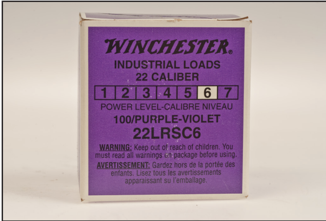
Figure 4-6—A box containing No. 6 power loads. This is the load that should normally be used to launch flares.
