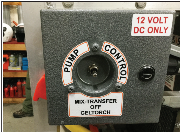
Figure 10–6—The terra torch control panel showing the three-way switch in the OFF position.
