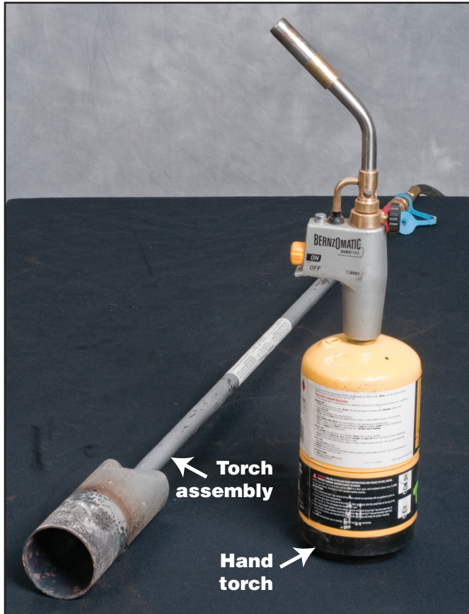
Figure 9-4—A small hand torch can be used to ignite a propane torch.
