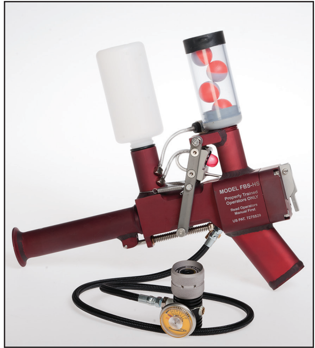
Figure 7–6—A newer version PyroShot HS plastic sphere launcher.
