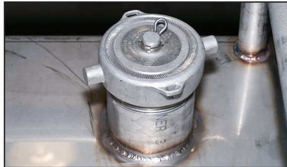
Figure 2-7 —A fusible cap for a fuel tank. If the tank catches fire, the cap will melt to prevent excessive pressure from building. Inspect the cap for cross-threading or damaged seals.
