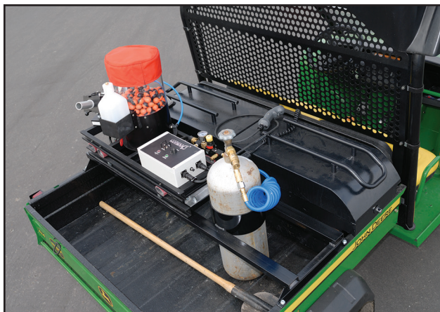
Figure 7–7—The SEI Green Dragon plastic sphere launcher mounted on a UTV.
