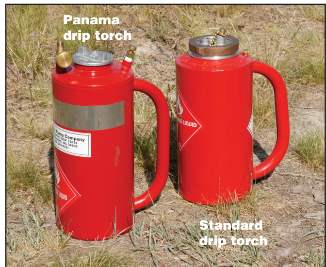
Figure 3–3—A Panama drip torch and a standard drip torch, both configured for transport and storage.
