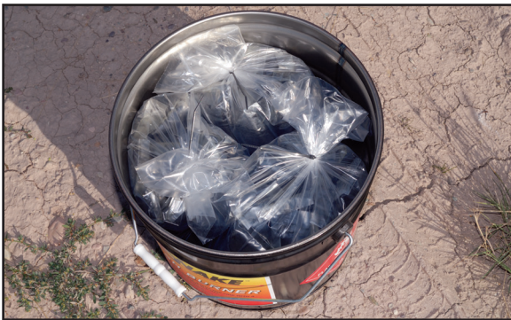
Figure 6-4—Put blivets inside a plastic bag before carrying them in the field.
