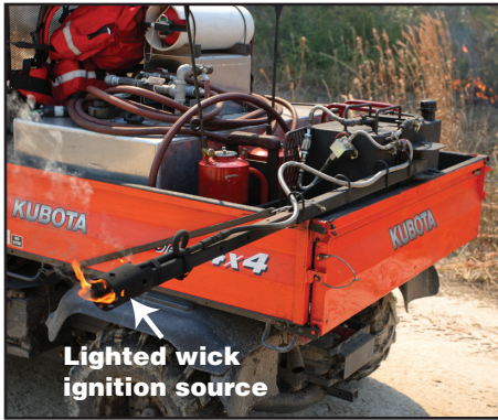
Figure 2–1—A UTV torch with a lighted wick ignition source. This UTV has a water tank and pump for fire suppression.
