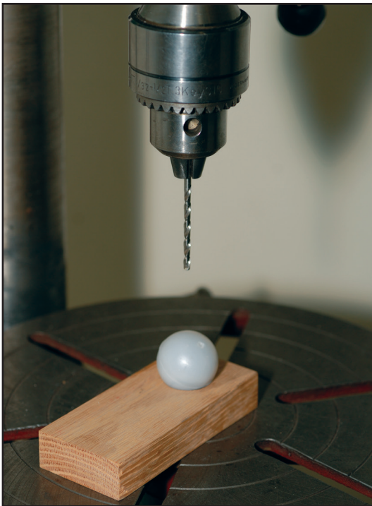
Figure 7–9—Support the sphere on a wooden block when drilling a hole so antifreeze can be injected.
