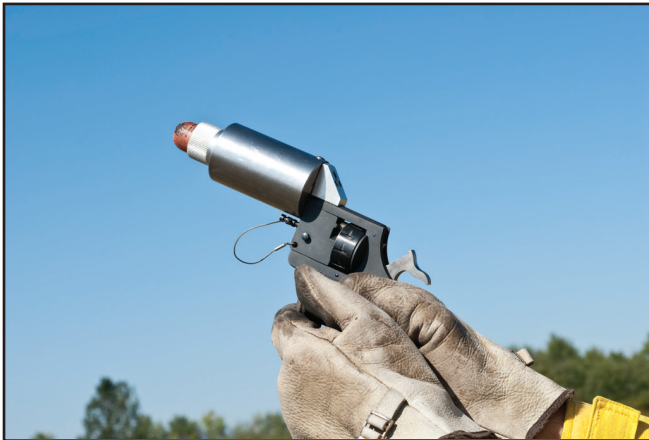
Figure 4–11—Launching a flare with the FireQuick flare launcher.
