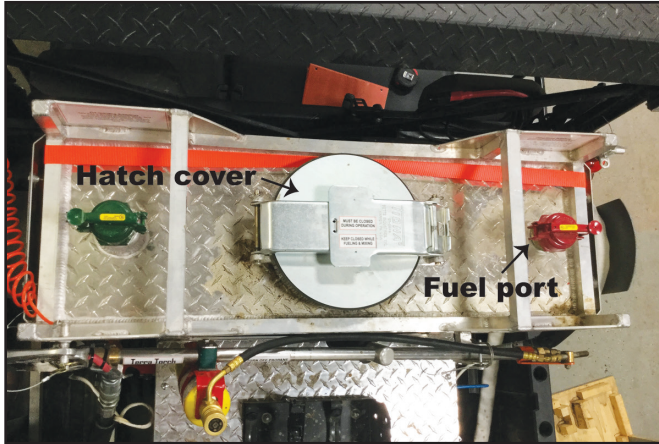
Figure 10–4—Fill the terra torch through the fuel port, not through the tank hatch cover, to avoid generating static electricity that could ignite fuel vapors.
