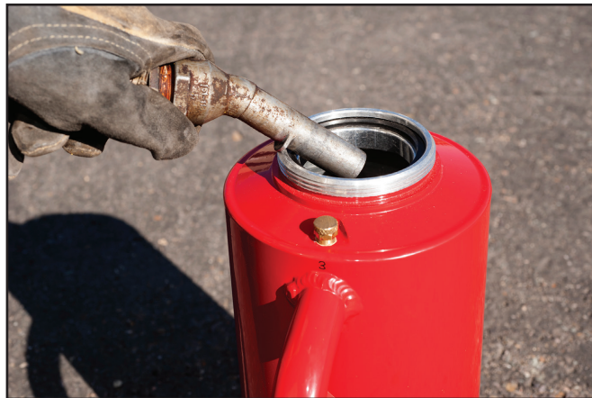
Figure 3–11 —Make sure that the pump or fuel container nozzle contacts the tank when filling a drip torch. Contact ensures electrical bonding, preventing static electricity from building up.
