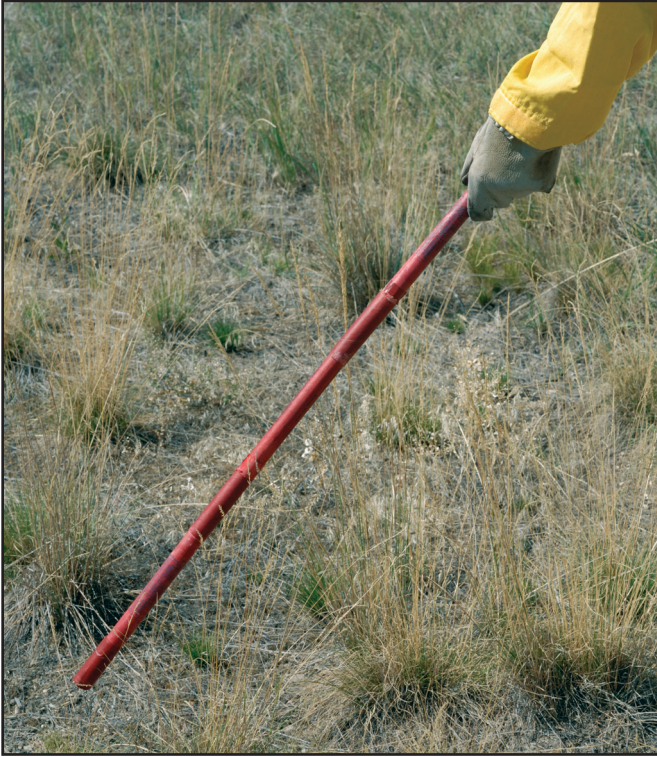
Figure 5-7—Several fusees may be joined together to form an extension handle to keep burning fusees away from your body.
