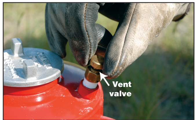
Figure 3–22—Open the vent valve of a Panama torch before use.
