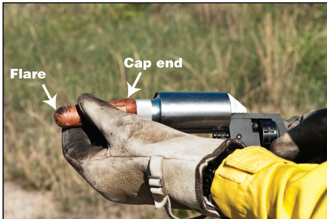
Figure 4-10—Loading a flare into the FireQuick launcher.
