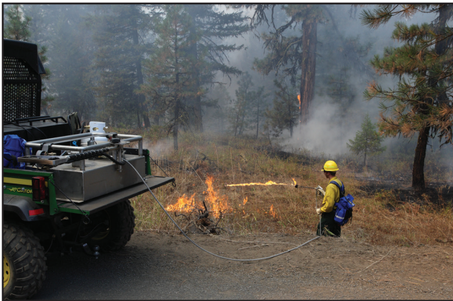
Figure 8–1—This power torch uses the same setup and components as a UTV torch, but the operator uses a handheld wand with an extension hose rather than a mounted wand.
