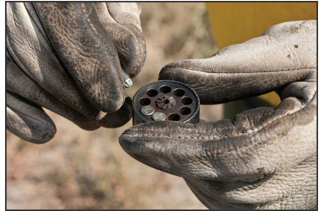
Figure 4-5—Insert power loads into the cylinder.
