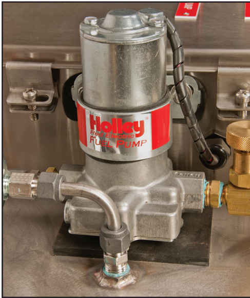
Figure 2-6 —Inspect the fuel pump for obvious damage and listen for correct operation.
