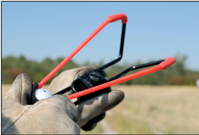
Figure 7–3—Slingshots may be used to launch plastic spheres.
