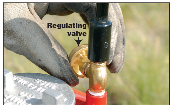
Figure 3–23—Adjust the regulating valve to control the flow of fuel.
