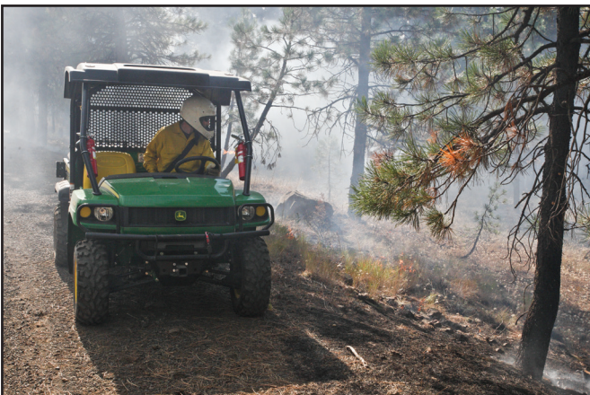
Figure 2–4—A UTV with brush guards, skid plate, and puncture-resistant tires. Fire extinguishers are mounted within the torch operator’s reach.
