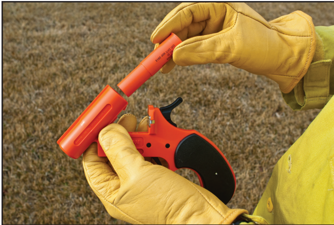
Figure 4-12—Loading an Orion flare launcher.
