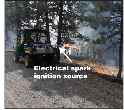
Figure 2–3—A UTV torch with an electrical spark ignition source.
