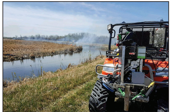
Fig 7–8—The Firecraft Products, Inc. Zinger mounted on the front receiver hitch of a utility-terrain vehicle.
